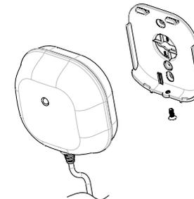
2. Unscrew the screw from the battery cover and remove the battery cover.
