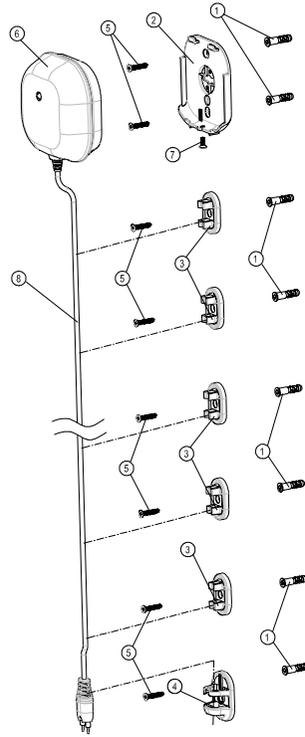
3. Fix the back cover, flood sensor cable rack and sensor rack using the fixing screws provided.
